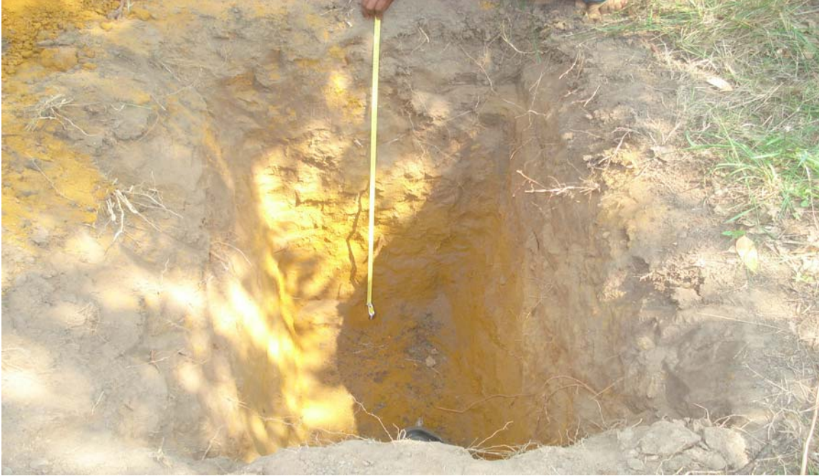
Figure 2: Measuring the depth of a soil horizon in a sampling pit
